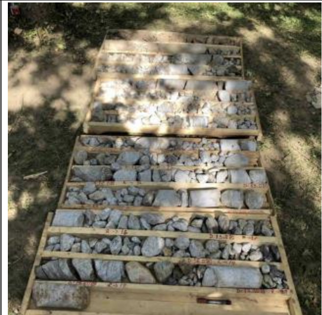
Photo 57: Drill cores at powerhouse
